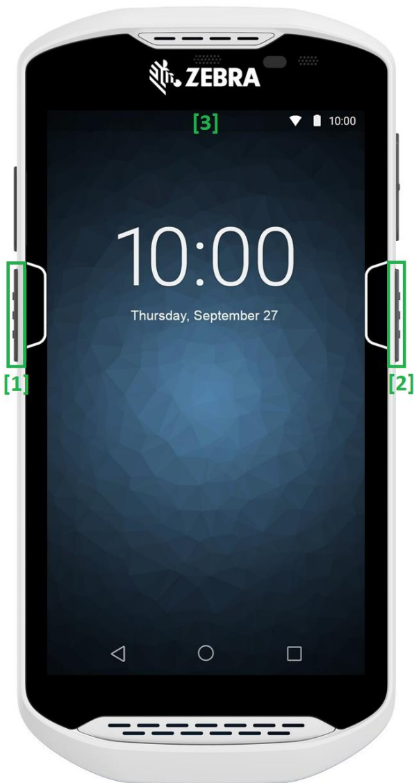
Figure 3: The Zebra-Scan is always triggered by pressing one of the three labeled hardware buttons. The third is on the back of the device.
