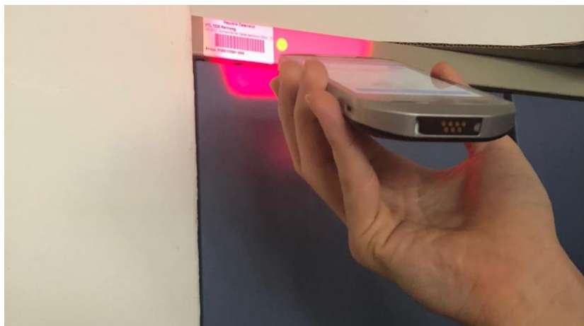
Figure 2: Zebra-Scan: This scan is triggered by hardware buttons and is only available on Zebra-Devices
